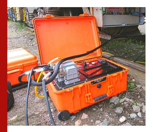
Portable Automeg is designed for testing in spaces too small for a standard rack-mount wire harness test system. It's easily deployable in the field for maintenance or repair fault finding.
